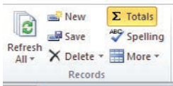
FIGURE 8.38 In Access, simple totals like sums and counts can be shown in queries by choosing the totals option.
