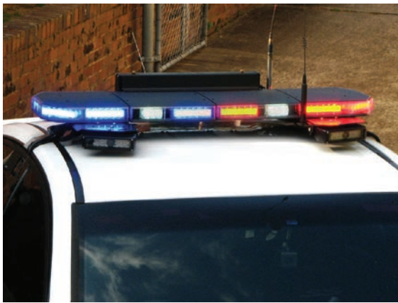
FIGURE 8.52 Roof mounted lightbar and ANPR cameras on a NSW patrol car
