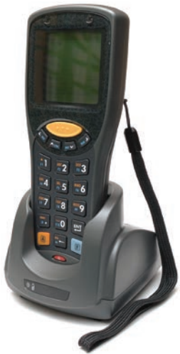
FIGURE 8.47 A data collection device that reads RFIDs and can communicate via wi-fi, Bluetooth and mobile phone network.
