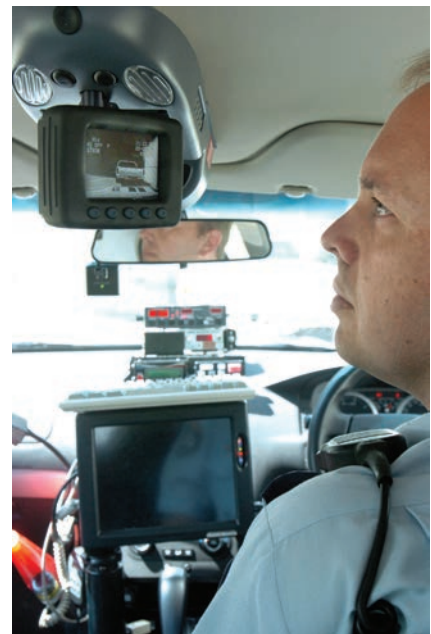
FIGURE 8.53 The ANPR terminal inside a police car
