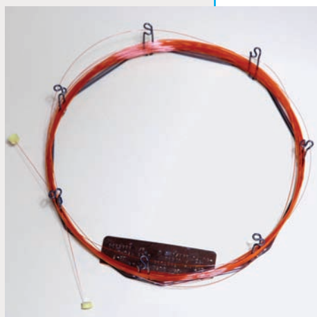
FIGURE 15.1 A typical capillary column for a gas-liquid chromatograph. This silica column is 30 m long with an internal diameter of 0.15 mm; the internal surface of the column is coated with the non-volatile liquid polydimethylsiloxane. This 'column' has been wound into a coil of about 20 cm diameter
