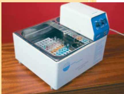
Figure 1.6 A modern bain-marie is used to heat solutions in a controlled way.
